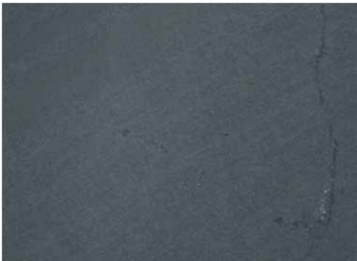
HONED: A smooth finish with a slight sheen, produced by using a polishing head.
