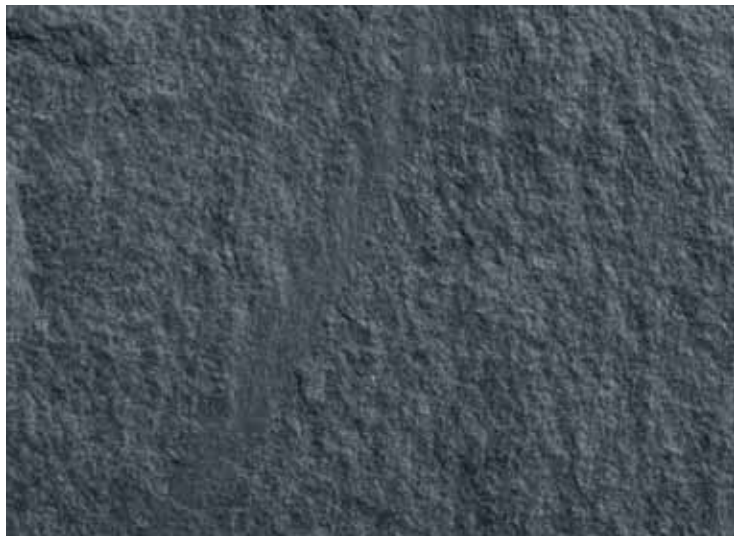
RIVEN CLEFT: A finish in which the stone is split along its natural cleavage plane.
