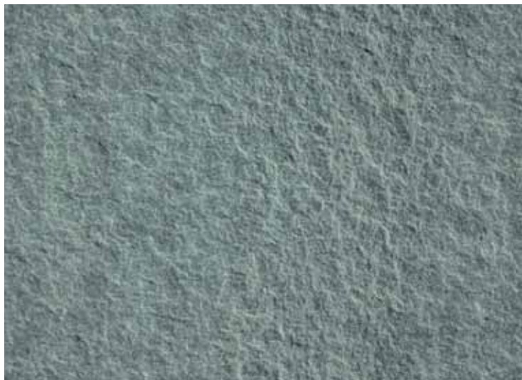
FLAME TEXTURED: Heat and water combine to achieve a regular textured finish.
