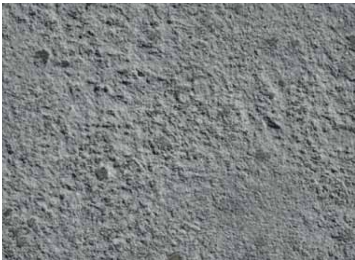
GRITBLASTED: A high-pressure airline projects coarse-grained abrasives, giving a regular non slip finish.
