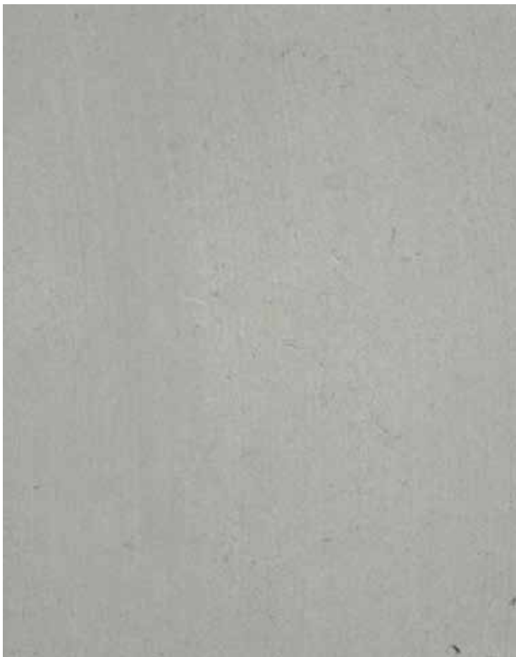
SANDED: The top surfaces of sawn slabs are coarsely diamond sanded to produce a non slip finish.
