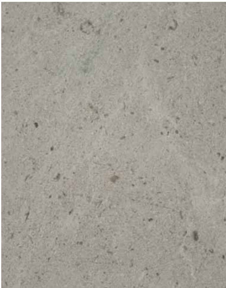
HONED: A smooth finish with a slight sheen, produced by using a polishing head.
