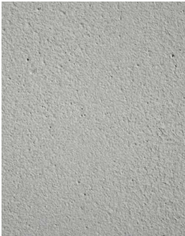
GRITBLASTED: A high-pressure airline projects coarse-grained abrasives, giving a regular non slip finish.
