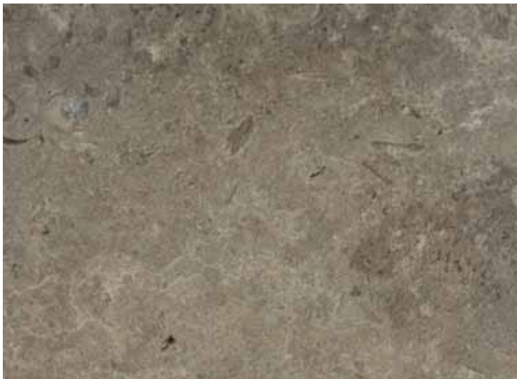
POLISHED: A smooth high gloss finish, produced by using a polishing head. For limestone only.
